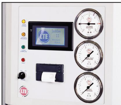
This system gives users a standard menu of porous load-specific cycles. This includes 121 and 134 cycles, both with the option of extended drying, plus leak rate test and Bowie Dick test cycles. The main load cycles can be adjusted to suit individual requirements.
