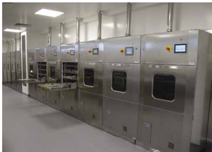
The ten Dekomed DEKO D32 Excel washer-disinfectors. The pass-through hatches can be replaced with further washer-disinfectors for future-proofing
